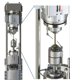
Figure 1: Axial+torsion rotating load train universal test system, incorporating spherical marker holders to measure axes rotation.
