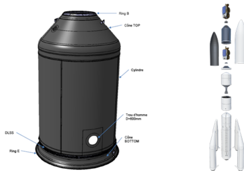
Figure 1: Ariane 6's Dual Launch Structure (left) and location within the launcher (right)
