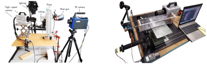
Figure 1: a) Thermography of jet impingement on titanium heated plate imaging setup b) Schlieren experimental setup
